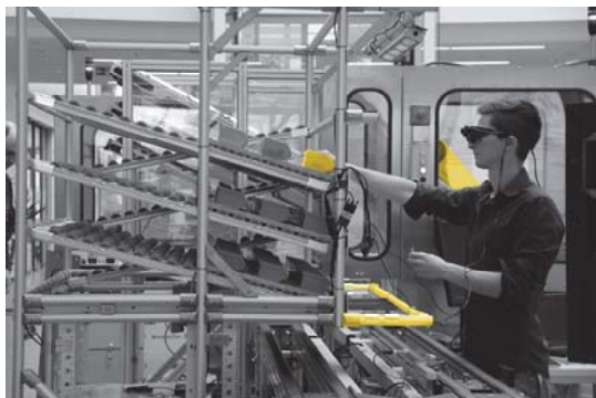
Assistance systems in the SmartFactoryOWL: An assembly instruction is projected onto Augmented Reality glasses.
