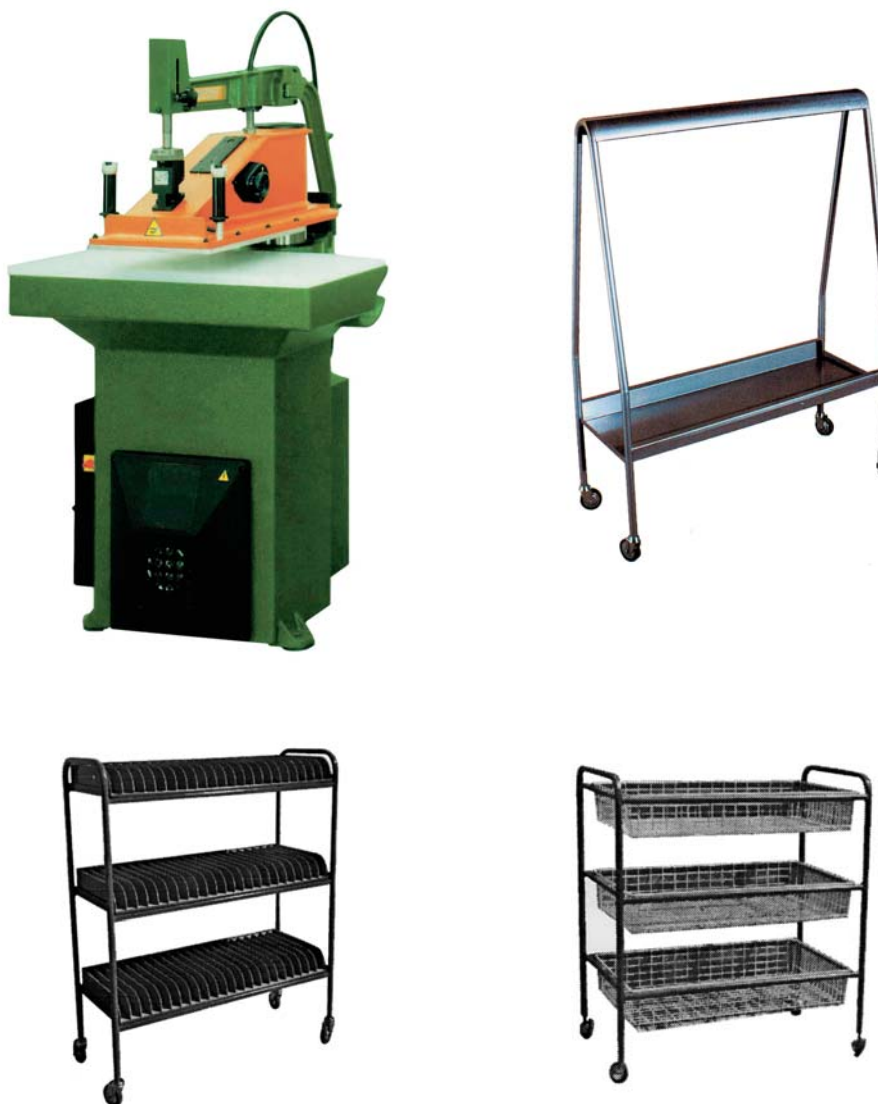
Picture 30 - Up: example of arm-type clicking press and leather holder trolley. Down: example of three-shelf last holder trolley, on the left; and upper holder on the right.
