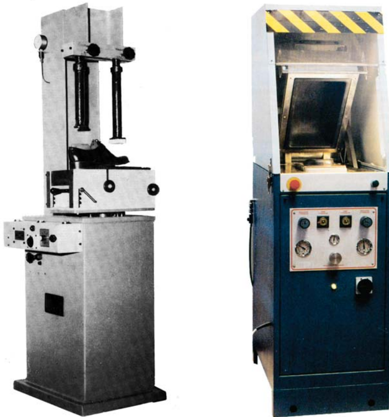
Picture 53 - Example of one station attaching machine for soles. Left, oleo-dynamic version with sectors' support; Right, pneumatic version, diaphragm-type, also suitable for opanka soles.
