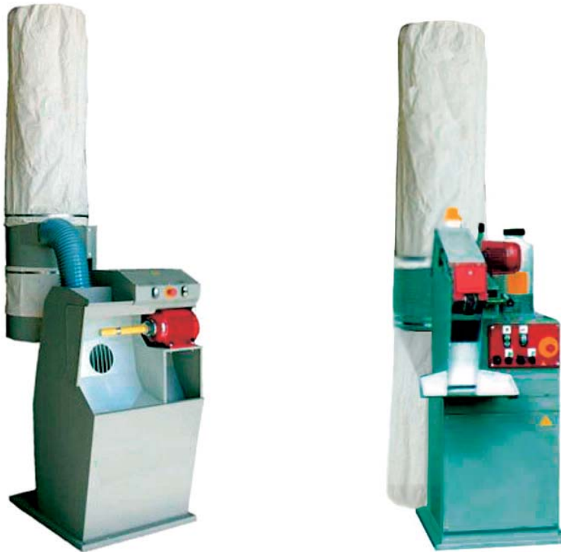
Picture 51 – Example of scouring machines for upper lasted edge surface. On the left, version with pad sandpaper; on the right, version with tape sandpaper.
