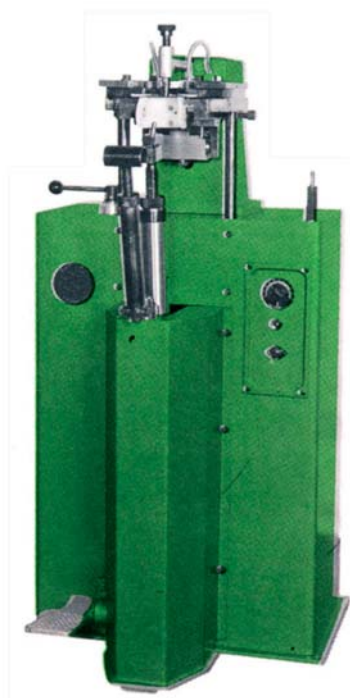
Picture 48 – Example of seat laster activated by compressed air.
