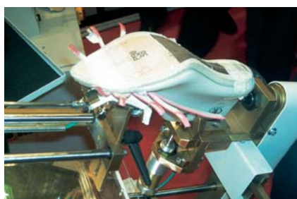
Picture 50 – Semiautomatic sandal sequential modalities. In the middle, insole's blocking system with mechanical arm.
