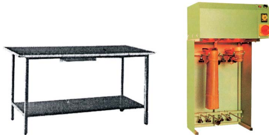
Picture 52 – Example of workbench for cementing the bottom of lasted shoe and sole and cement reactivation heater.
