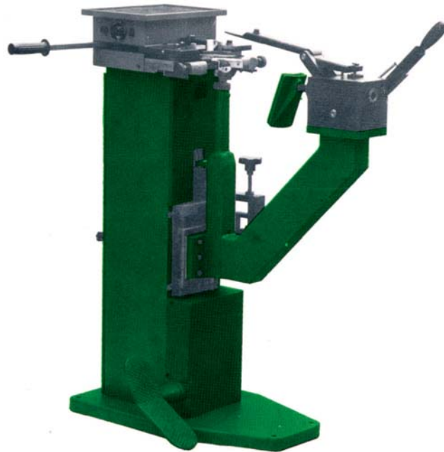
Picture 47 – Example of pneumatic toe laster.
