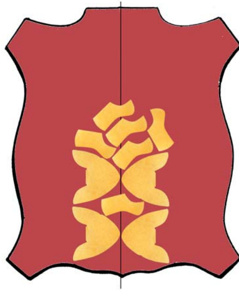
Picture 28- Example of templates' correct arrangement on leather.
