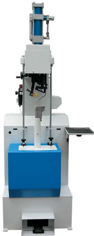
Picture 59 – Example of heel nailing machine with delicate interventions of efficient tightness.
