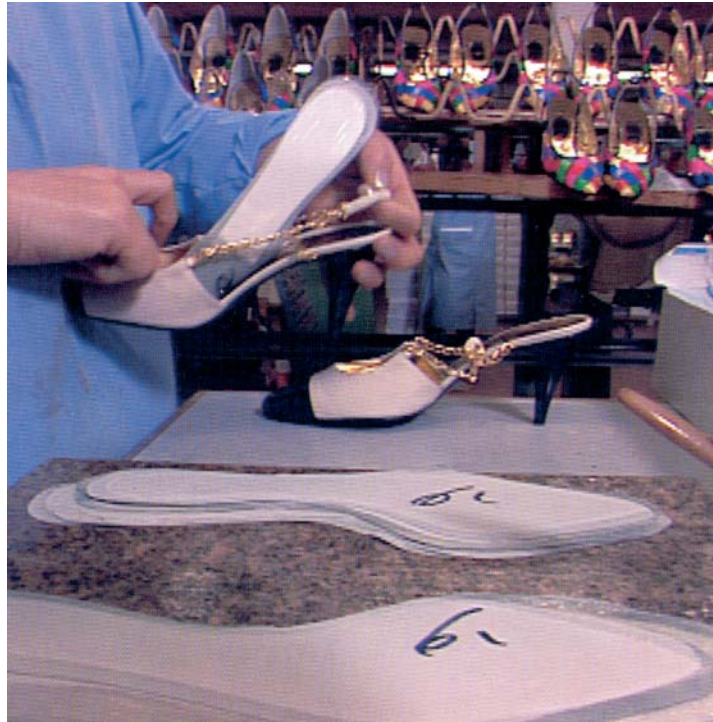
Picture 65 – Example of cleaning board shank application.
