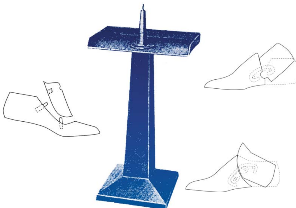
Picture 56 – Example of equipment for the support of the lasted shoe during last pulling and last arrangement manners before the intervention.
