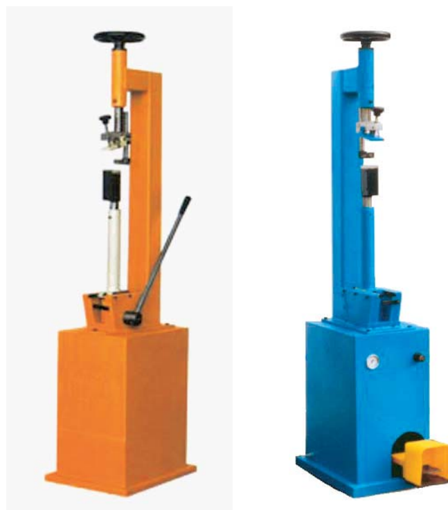
Picture 58 – Example of heel nailing machine: the first one on the left is the manual version; the second one on the right is the pneumatic one.
