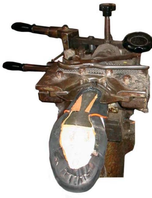
Picture 46 – Seat lasting with machine worked by hand.
