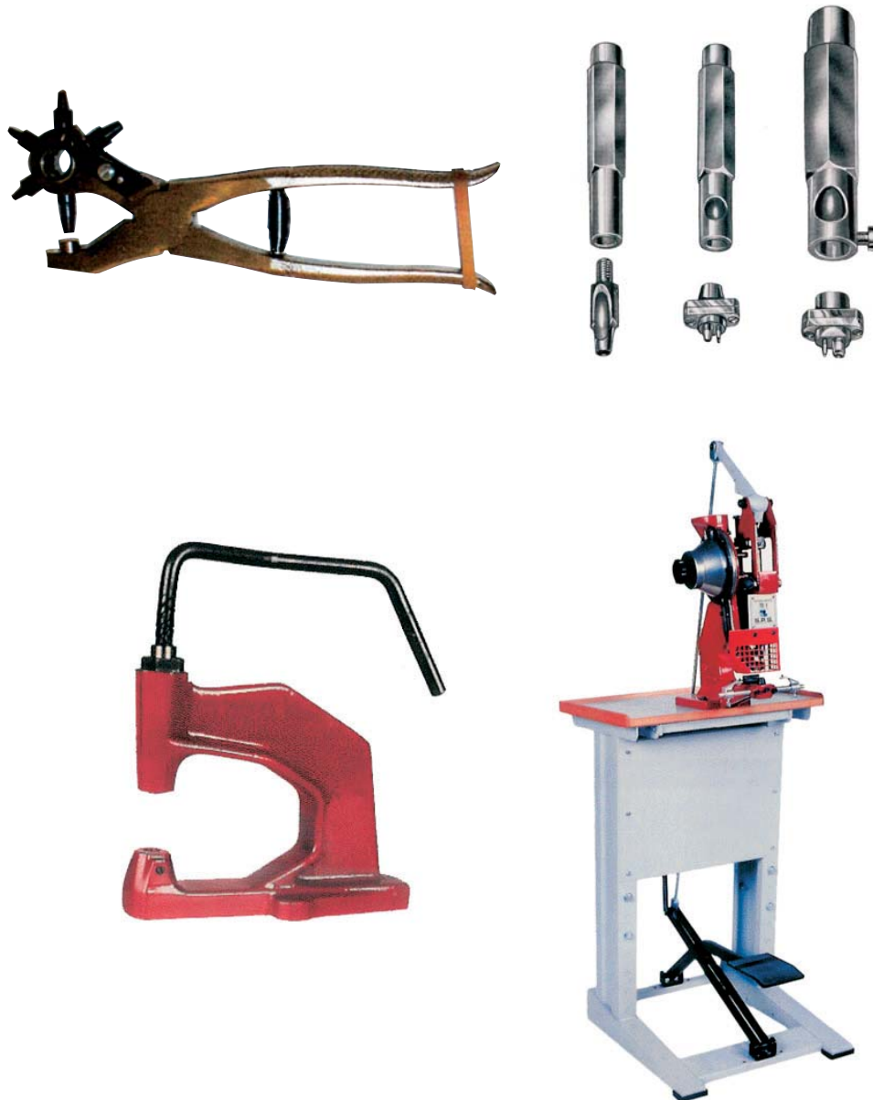
Picture 40 - Up: other manual tools for the stitching department. Down: Equipments for the application of small metallic articles in general: completely manual on the left; first mechanization on the right; with materials' perforation and contemporary application of the small metallic article.
