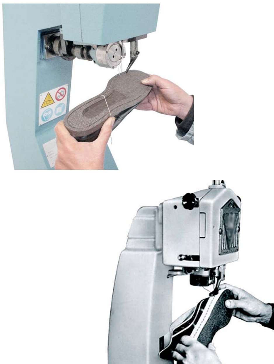
Picture 57 – On the left, example of shoe bottom Blake sewing machine; on the right, sole side stitching.
