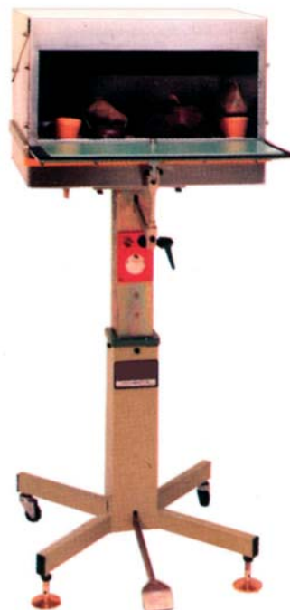
Picture 44 - Example of equipment for upper humidification and reactivation of toes and stiffeners.
