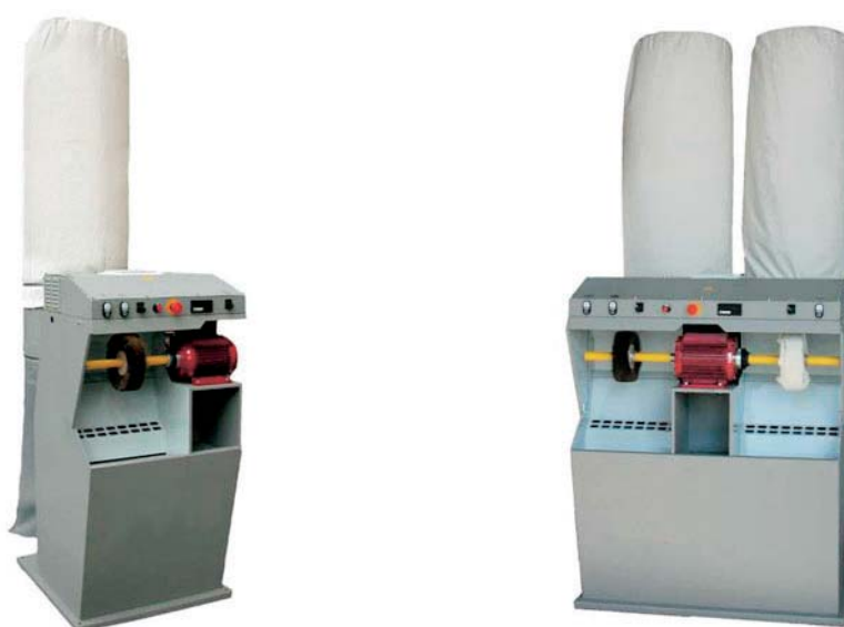
Picture 68 – Example of brushing-polishing machines with one station on the left and two on the right.
