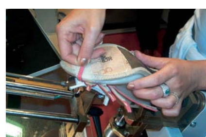
Picture 50 – Semiautomatic sandal sequential modalities. In the middle, insole's blocking system with mechanical arm.
