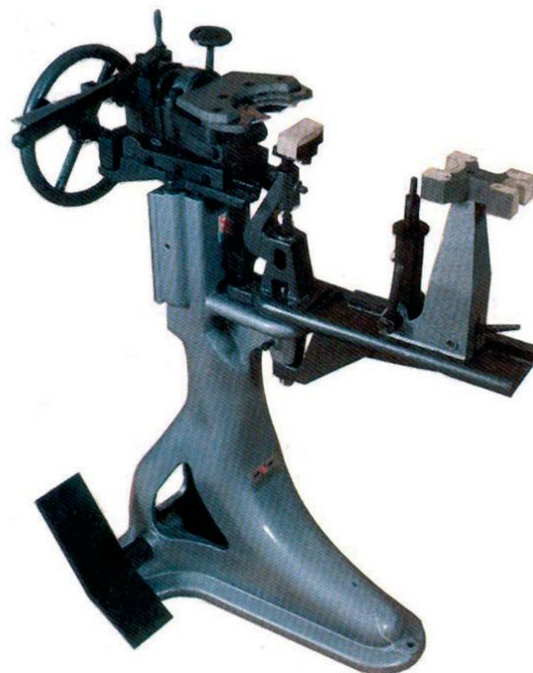
Picture 45 – Example of toe and seat laster used in artisan structures.
