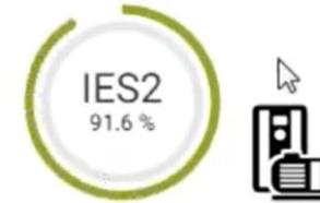
System efficiency determined according to EN 50598 - 2 and IEC 61800-9
