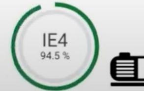
Motor efficiency determined according to IEC 60034-30-1
